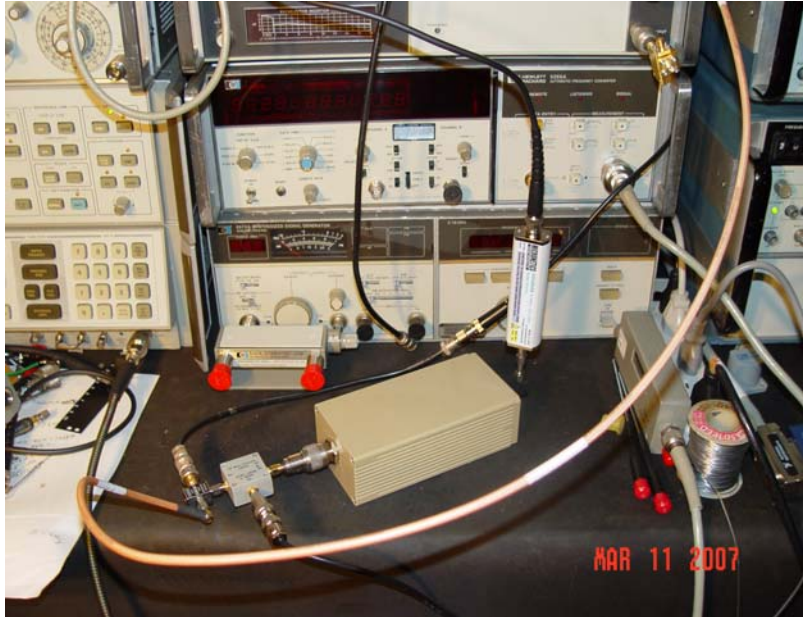
FIGURE 2. TYPICAL TEST SETUP AT EOZ WITH Cont.'S MICRONETICS NOISE SOURCE AND Man. LNB
